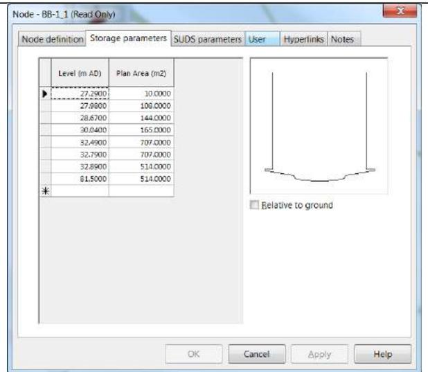
Figure 10 – Shaft BB-1 following manual correction and representation of shaft benching
