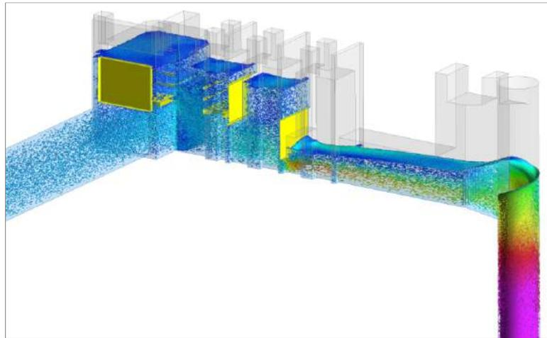
Figure 7 – CFD Modelling of Vortex Drop Connection
