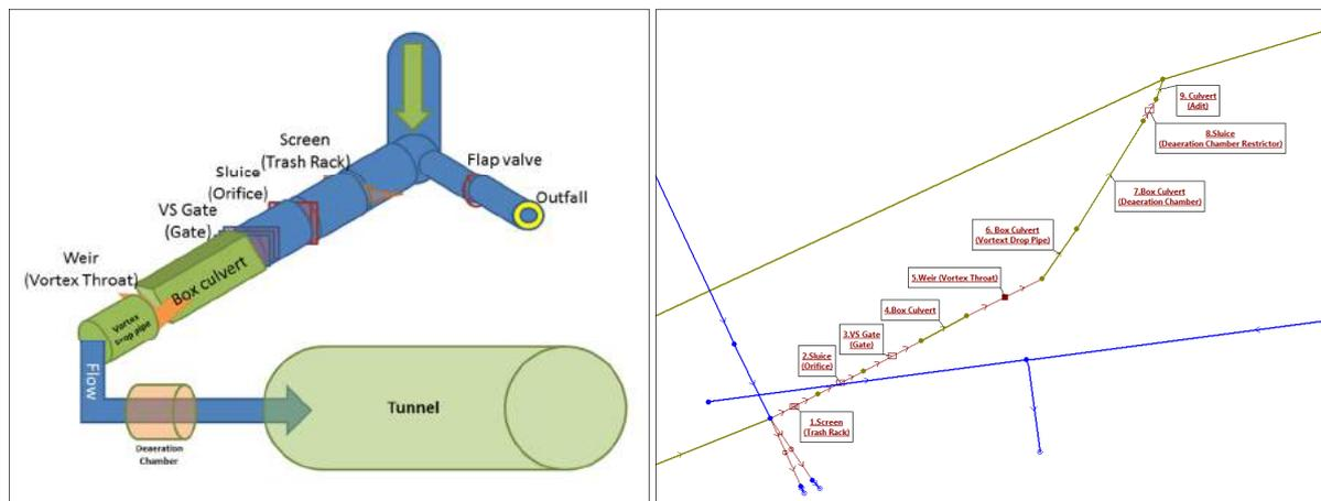
Figure 5 – Schematic and Modelled Representation of Vortex Drop
