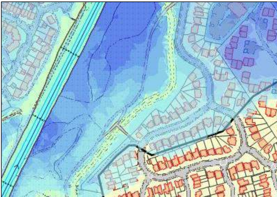
Figure A4-3: Visualisation of Simulated Flooding compared to recorded flood outline
