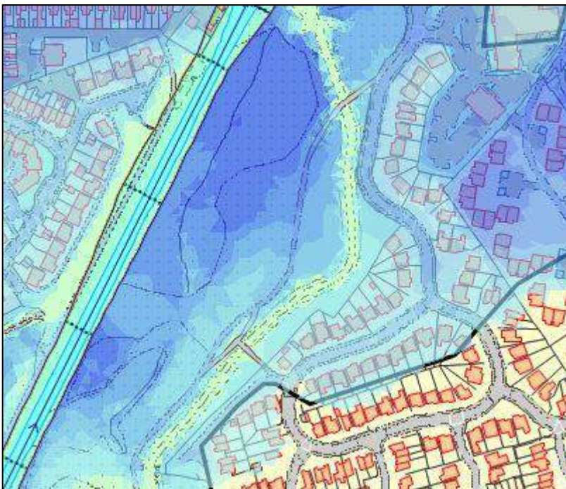
Figure A6-1: Example of 2D flooding verification
