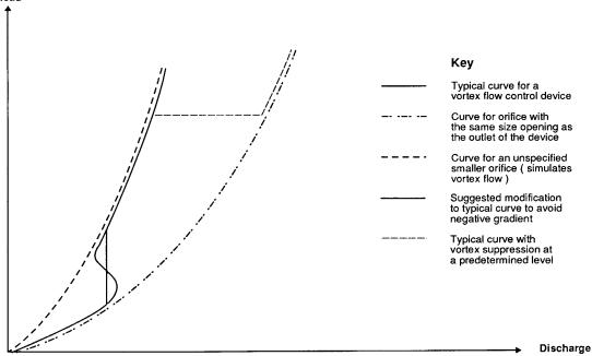
the device. At low heads the vortex will collapse and the characteristic will revert to that of the larger orifice. This will also occur if there is a negative head across the device. With high heads upstream of the device the vortex remains but with increased air pressures inside the core. This reduces the operating head to the differential head across the unit.
